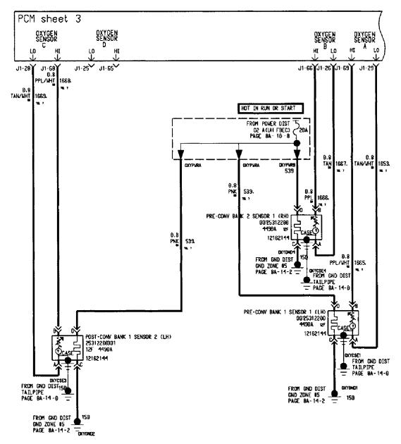
NOTE: P/N'S & CONN'S SHOWN ABOVE FOR PRE-CONV 02 SENSORS ARE FOR L35 LD L35 HD 02 P/N'S - PRE-CONV BANKS 1&2 P/N 225312191 CONN NO 12162102 POST-CONV P/N'S & CONN'S ARE FOR ALL L35
